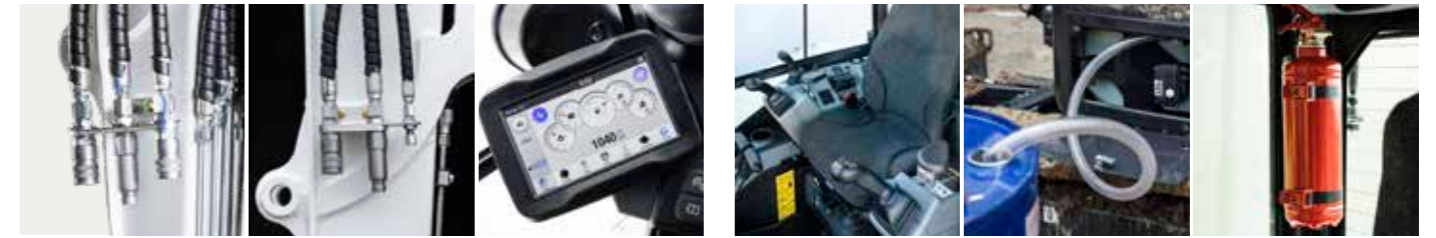
1st AUX hydraulic on arm 2nd AUX hydraulics w/ drain line 7-inch display Dlx textile suspension seat Electric re-fill pump Fire extinguisher
